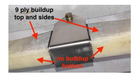
total width of the layup including all ply drops will be  $\sim$ 6 ½". The easiest way to accomplish this is to do the layup on 4-mil poly sheet, starting with a 2.25" wide strip, then increasing the width of each strip by ¼". Then wrap this layup on the strut, trim the ends so they don't extend onto the bottom surface, and peel ply and let cure.
